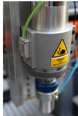
Fig. 6. Machine spindle and the surface where MEMS sensor is mounted
